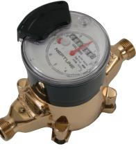
Every T-10 water meter meets or exceeds the latest AWWA C700 Standard. Its nutating disc, positive displacement principle is time-proven for accuracy and dependability since 1892, ensuring maximum utility revenue.
