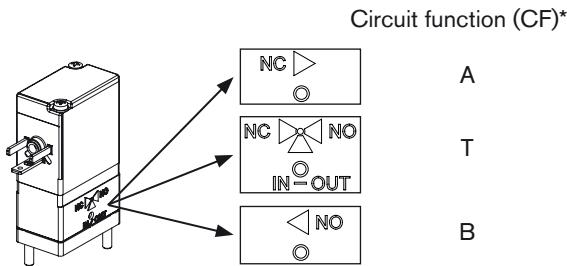
Identification of the valve connections on the body:
