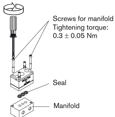
→ Insert the seal into the valve.
