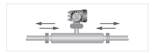
Mass flowmeters have a maximum level of force (negative or positive) that can be applied to the ends of the meter. Refer to the table below for permitted forces.
