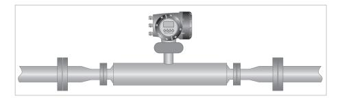
Always avoid extreme step changes in pipe size. Use pipework reducers, where there is a large difference between pipework size and meter flanges.
